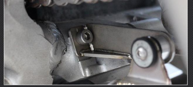
**15)** Now take a good look all around and check for interference issues with the frame, swingarm, cowling etc. The routing of the pipe does have a little adjustability by a bit of twisting here and there.
