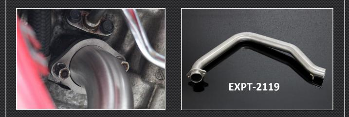
7) Fit the rear left header pipe (EXPT-3119) and secure with the spring.
